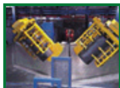
Once tanks are filled with PermaGlas, they are rotated (computer controlled) for precise, even coating.
